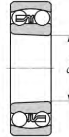
Tapered bore taper 1:12
