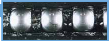
Detail view of the ball cage
