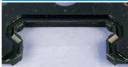
Lip has not been fractured
