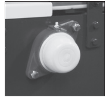
Safety end caps protect against rotating stub shafts.
