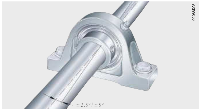
Figure 1 Compensation of static shaft misalignment
