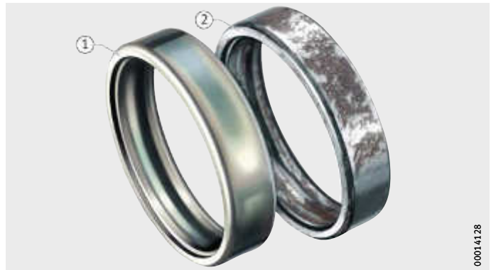
Figure 7 Bearing rings after the salt spray test
