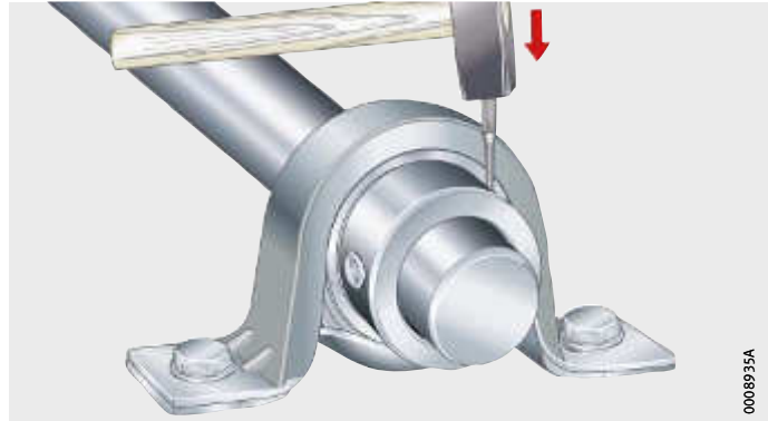
Figure 13 Tensioning the eccentric locking collar
