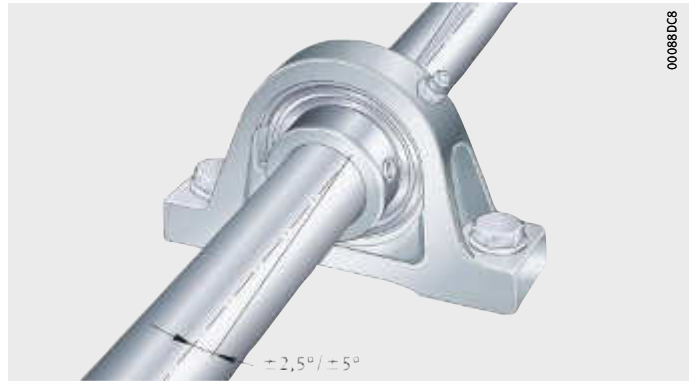
Figure 1 Compensation of static shaft misalignment
