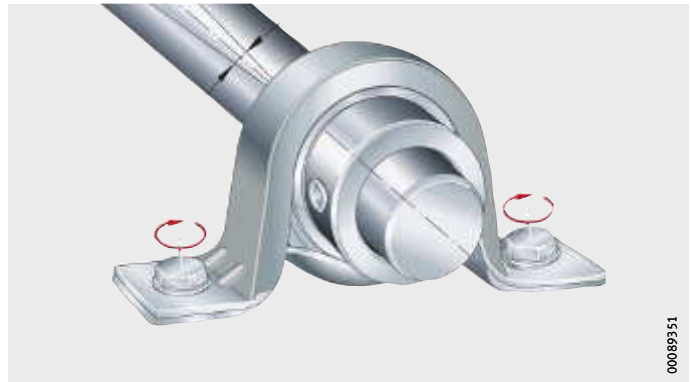
Figure 12 Screw mounting the housing finger tight
