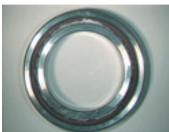
Photo. 6.1 Filling grease into angular contact ball bearing
