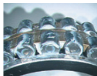
Photo. 6.2 Filling grease into cylindrical roller bearing
